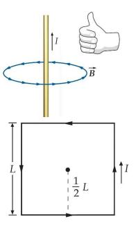
Example: The current is 1.7 A. Find the magnetic field at y = 6 cm on the y-axis.
