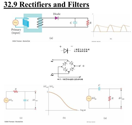
Low Pass Filter – High Pass Filter
