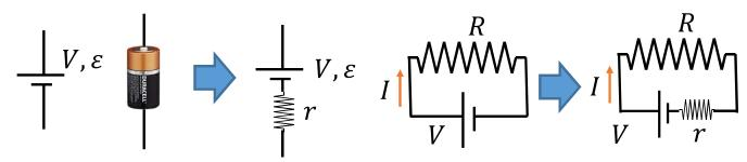
The electrochemical cells have internal resistors originating from chemical reactions and flow of ions.
