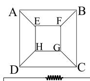
The points E and D are equipotential. The points F and C are equipotential.
