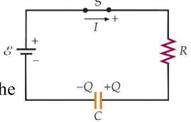
The battery provided energy will be stored in the capacitor and consumed in the resistor.
