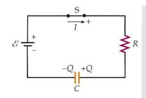
$$R\frac{dQ}{dt} = \varepsilon - \frac{1}{C}Q \to \frac{dQ}{C\varepsilon - Q} = \frac{1}{RC}dt \to -\int_{0}^{Q(t')} \frac{d(C\varepsilon - Q)}{C\varepsilon - Q} = \int_{0}^{t'} \frac{dt}{RC}$$
