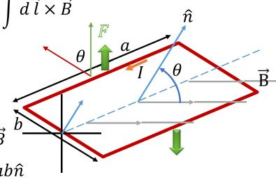
Lorentz Force on a Current Loop, Magnetic Moment, Torque, Potential Energy
