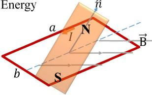
Determine The Polarity of Charged Particles and The Carrier Concentration
