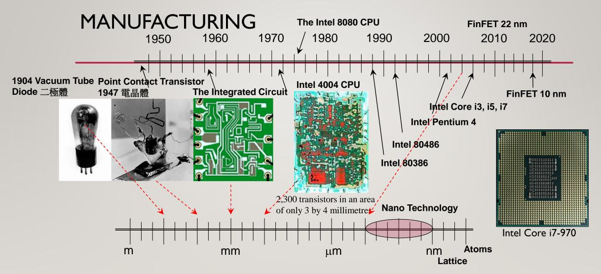
Making a transistor as small as possible is the way to assemble more transistors in the CPU. The final size of materials with periodic lattice structures is nano meter. That could be the smallest size while maintaining thermal stability for making electronic devices.
